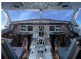
The cockpit of the Airbus A330-200. The interaction between man and machine in the last two decades has moved toward computers flying the jet, with pilots more at the receiving end of electronic commands rather than the other way around. Source: Airbus via Bloomberg News.
